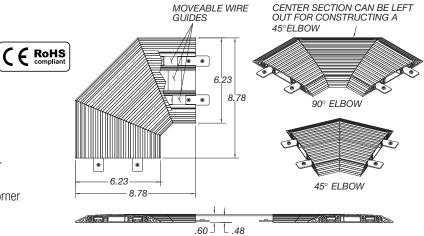
Moveable wire guides are provided with the raceway.
